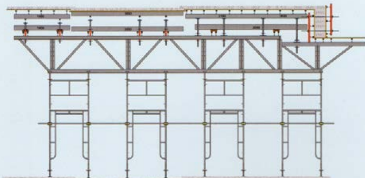
Layout of Table Form on Scaffolding Supports
