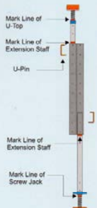
Figure B: Jack and Extension Staff Leg Markings
